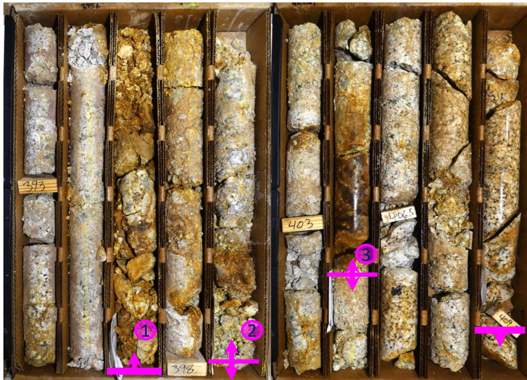
Qtz-iron oxide veinlets in faulted and brecciated Cambro-Ordovician Crowded Porphyry
